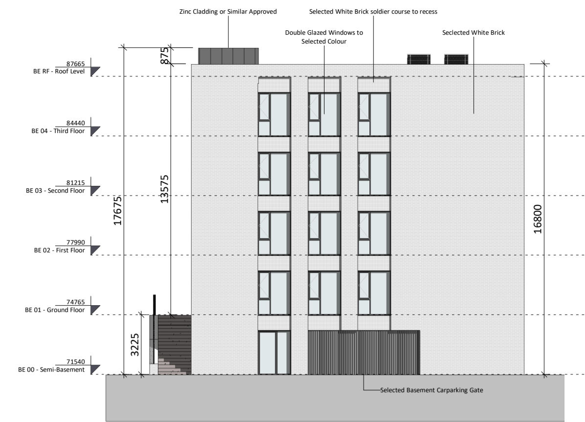
2 Block E North Elevation 1 : 200
